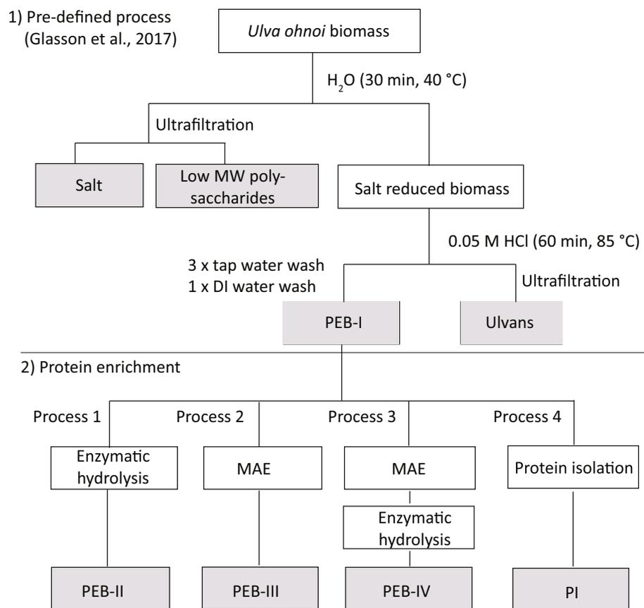
**Fig. 1.** Flow chart of biorefinery process options 1–4 using enzymatic hydrolysis (process 1), microwave-assisted hydrolysis (MAE; process 2), a combination of these methods (process 3), or protein isolation (process 4) to generate high-concentration protein products. Shaded boxes represent potential or alternative product streams. MW, Molecular weight; DI, deionized water (milli-Q); PEB, protein-enriched biomass; PI, protein isolate.
