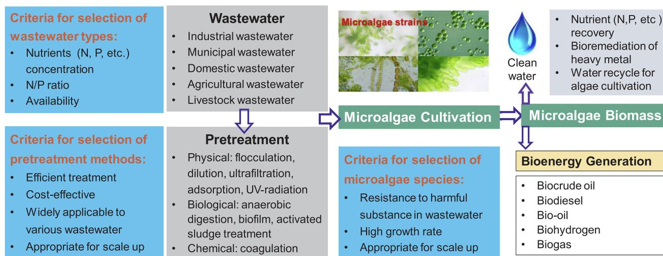
Fig. 1. Main processes from wastewater to algae cultivation and biofuel generation.
