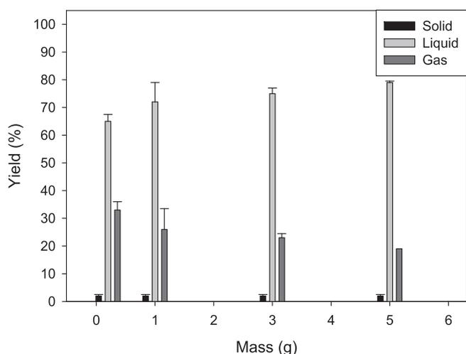
Fig. 4. Product yields for *Botryococcus braunii* pyrolysis at 500 °C changing biomass quantity. Values correspond to mean  $\pm$  standard error (n = 2).
