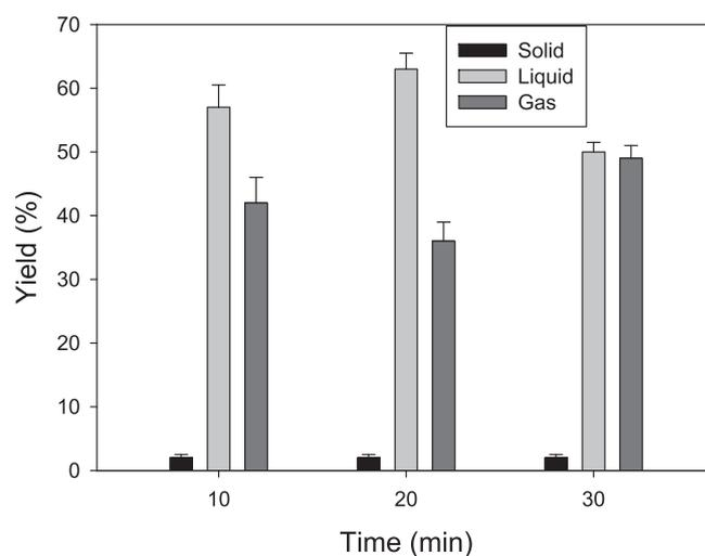
Fig. 3. Product yields for pyrolysis of *Botryococcus braunii* at 500 °C evaluating different reaction times. Values correspond to mean  $\pm$  standard error (n = 2).
