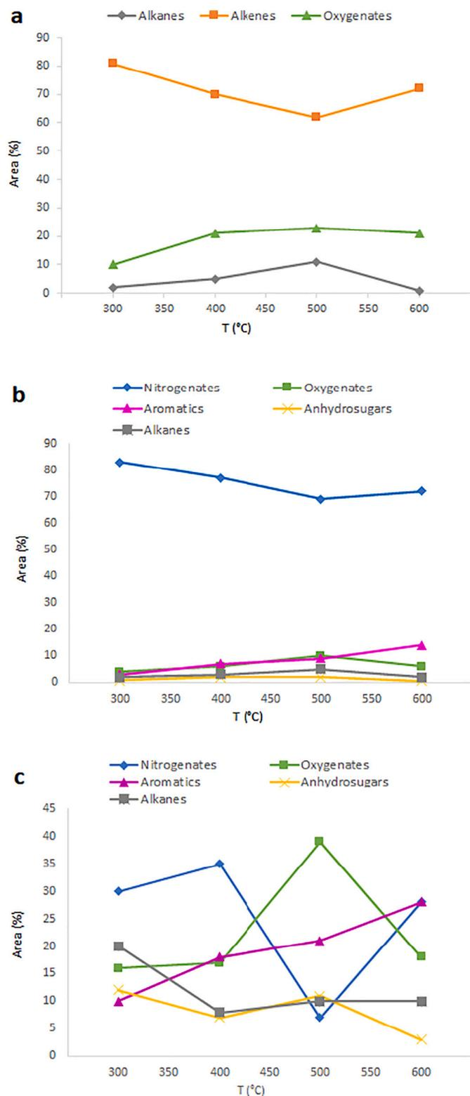
**Fig. 1.** Composition of bio-oils: a) from pyrolysis of *Botryococcus braunii*, b) from pyrolysis of *Spirulina platensis* and c) from pyrolysis of *Pithophora* sp. Values correspond to the mean  $\pm$  standard error ( $n = 2$ ).
