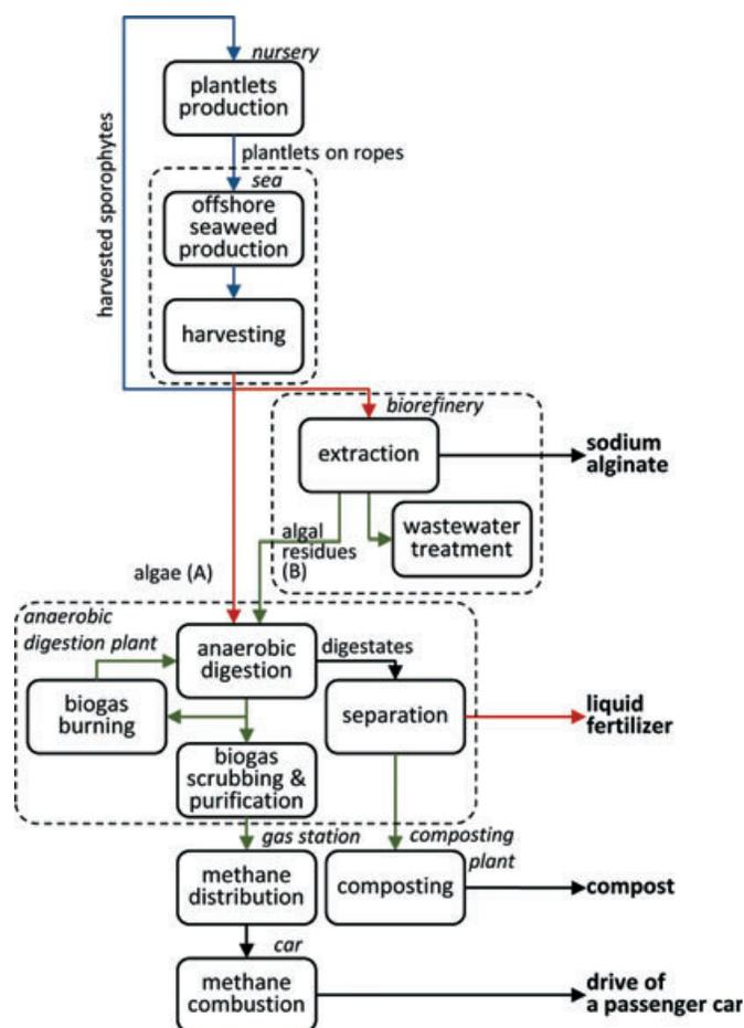
Figure 1. Overview of the biomethane production system (A) from whole seaweeds cultivated in the open ocean and (B) from residues of alginate extraction. Blue, red and green arrows stand for transportation by boat, truck and pipe respectively.
