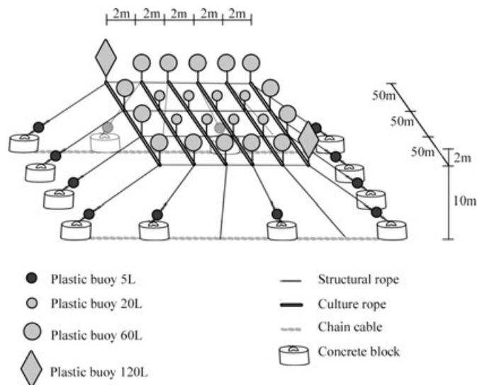
Figure 2. Schematic representation of a long-line raft.
