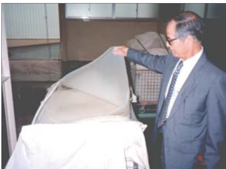
FIGURE 11 A sheet of agar gel after squeezing in the dewatering machine.
