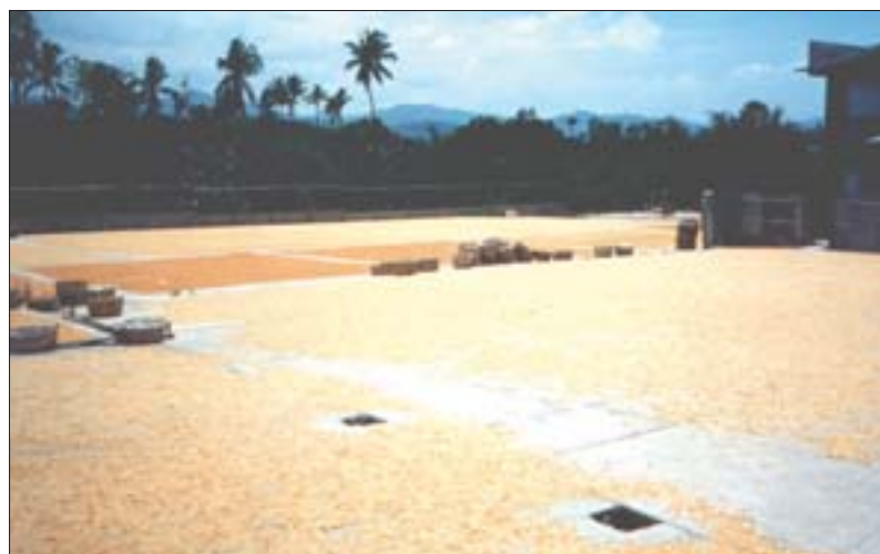
FIGURE 44 Sun drying semi-refined carrageenan (alkali treated K. alvarezii ).
