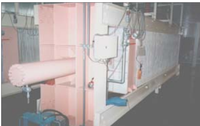
FIGURE 10 Dewatering machine used to squeeze water from agar gel.
