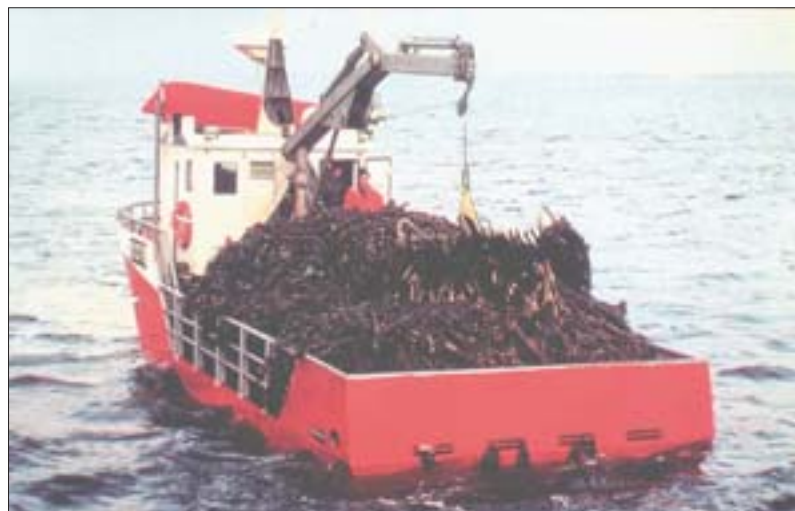
FIGURE 30 Harvesting Laminaria hyperborea in Norway. The crane has just lifted aboard the rake and its load of seaweed. Prongs of the rake are visible on the right-hand end.
